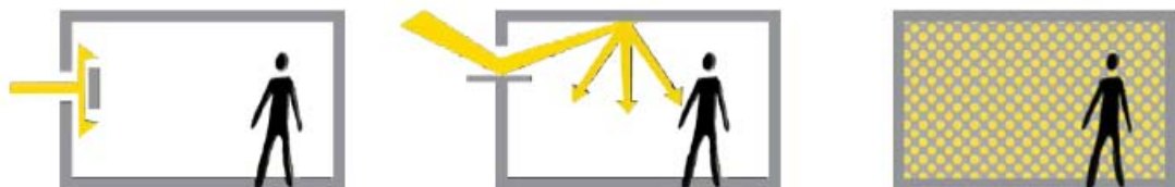
Figure 1 – Three different concepts for direct natural light: directing to the wall, directing to the ceiling and a light-through wall
